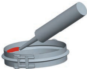
Figure 6 - Joint Assembly Step 1
