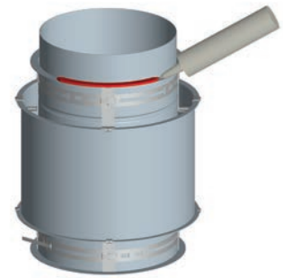
Figure 7 - Joint Assembly Step 2
