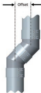
Figure 36a - Offset of two elbows
