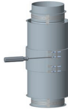
Figure 11 - Joint Assembly Step 6
